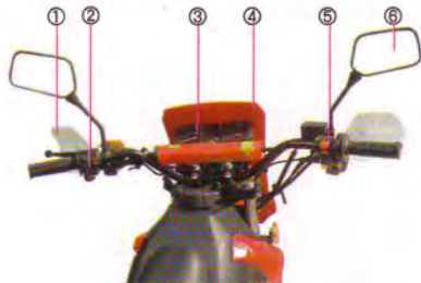
Fig. 3 ① Hand guard ② Left handlebar controls ③ Meter and indicator ④ Front fairing ⑤ Right handlebar controls ⑥ Rear-view mirror
