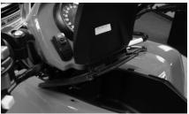
Lift out the storage box; then unsnap the four spring-clips and remove the air filter cover.
