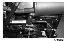
The ESN is located on the left-side of the engine crankcase.
