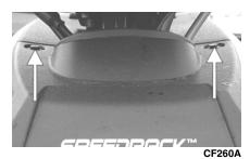
2. Lift up on the rear of the steering post cover and slide the storage compartment cover assembly forward to disengage the mounting lugs; then lift and remove the cover assembly from the storage compartment.
