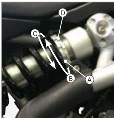
therefore make the suspension softer, turn the adjustment ring nut "A" in direction (C). At the end of the adjustment, tighten the return ring nut (D).
