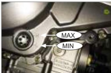
the oil as described in the section “Topping up the engine oil”. We recommend using *Petronas Power Speed 4T* oil
