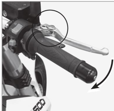
The brake lever has a position adjustment knob "1". To adjust the distance between the brake lever and the accelerator dial, turn the knob clockwise or anticlockwise; anticlockwise will move the lever closer, while clockwise will move it further away. Make sure that the correct adjustment, set from the adjustment gauge, is in line with the brake lever reference "2".
