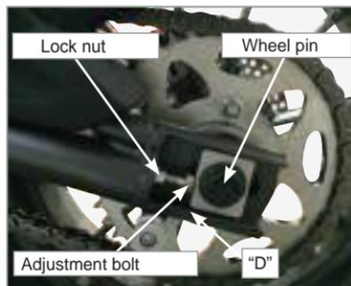
4. If the chain tension is not correct, adjust it as follows.
