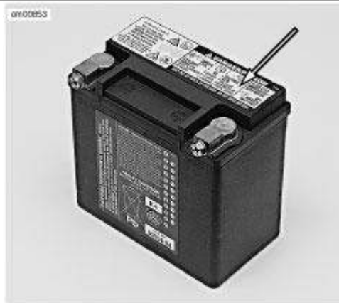
Battery Warning Label
