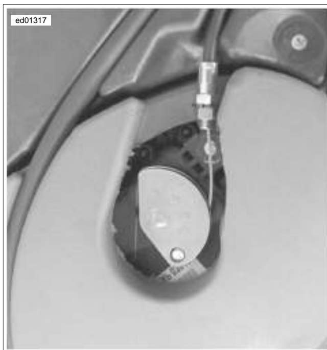
Figure 2-98. Active Muffler Control Actuator (Closed)
