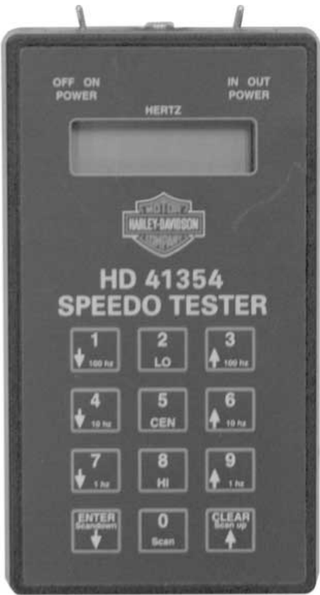
Figure 2-61. Speedometer Tester (Part No. HD-41354)
