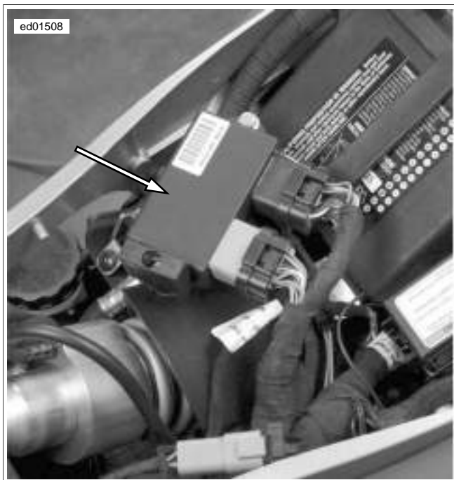
Figure 2-73. Electronic Control Module (Ulysses)
