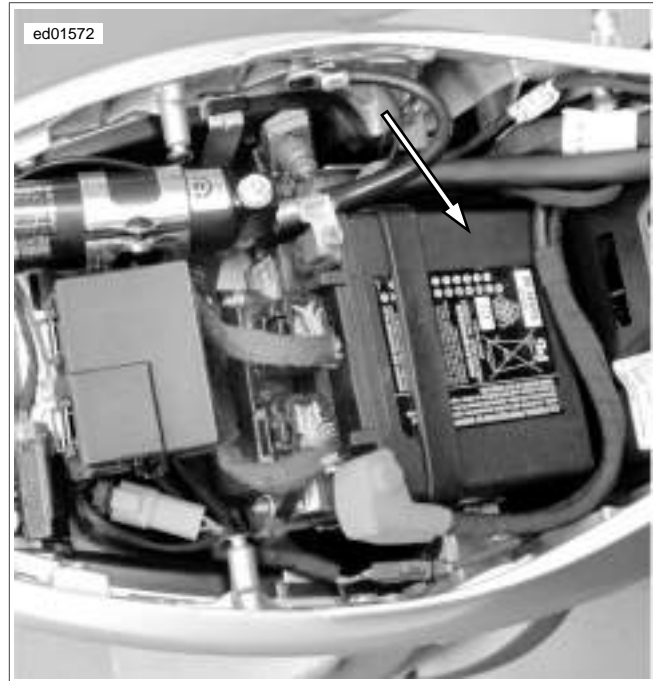
Figure 2-69. Battery Location (Lightning)
