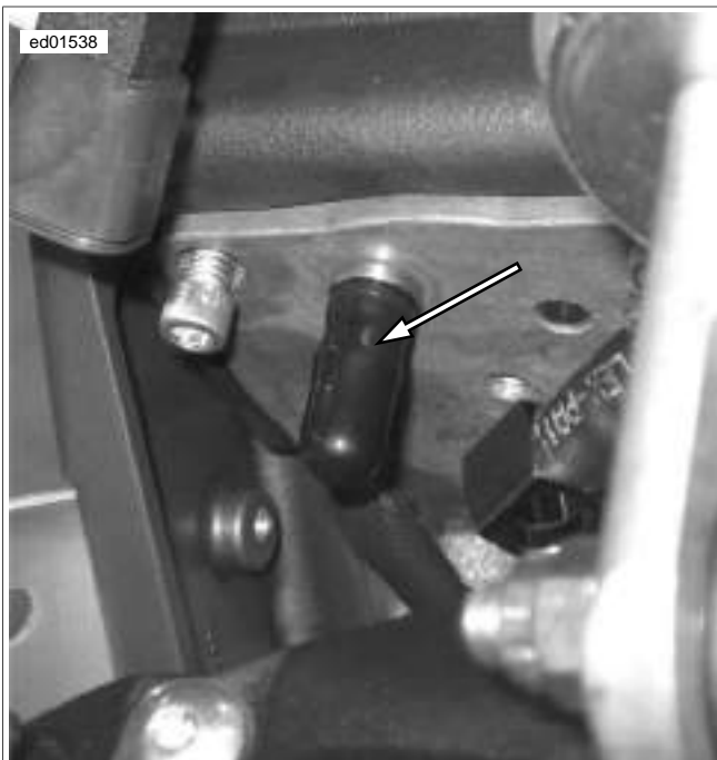
Figure 2-37. Fuel Pump Connector [86] (Firebolt - swingarm removed for illustration)
