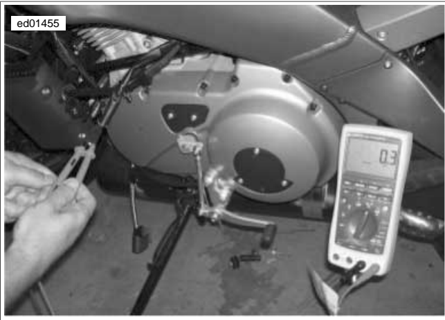
Figure 1-24. Check for Stator Resistance (Typical)
