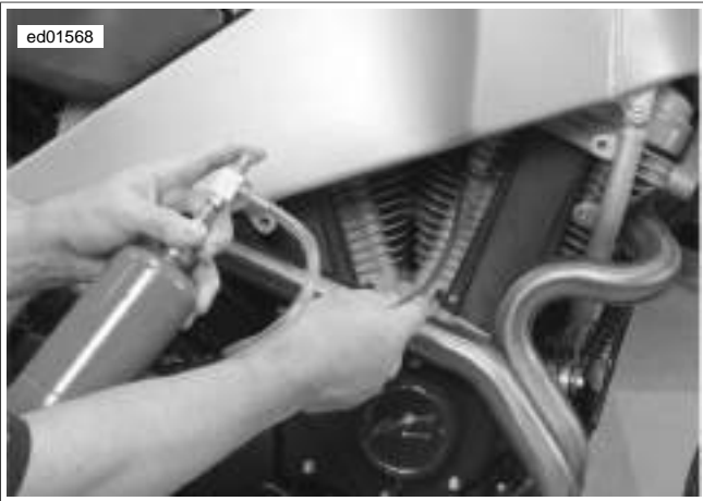
Figure 2-16. Checking for Leaks
