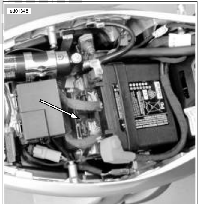
Figure 2-25. Electronic Control Module (Lightning)
