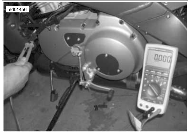
Figure 1-25. Check Stator AC Voltage Output (Typical)
