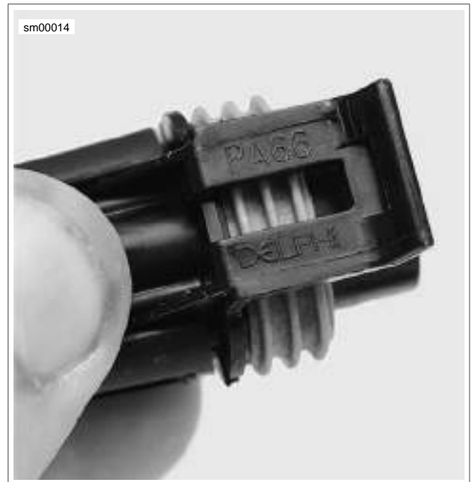
Figure A-8. Delphi Connector: Socket Housing Latch
