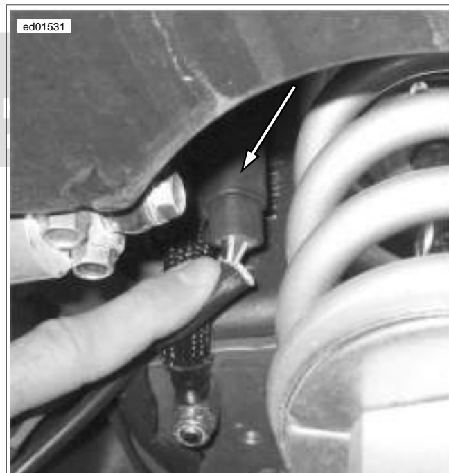
Figure 2-35. Fuel Pump Connector [86] (Ulysses - swingarm removed for illustration)
