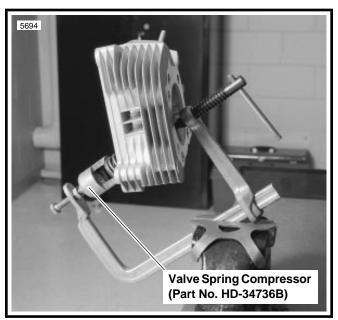
Figure 3-11. Compressing Valve Springs
