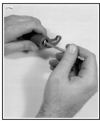
Figure 3-15. Measuring Rocker Arm Bushing Inner Diameter
