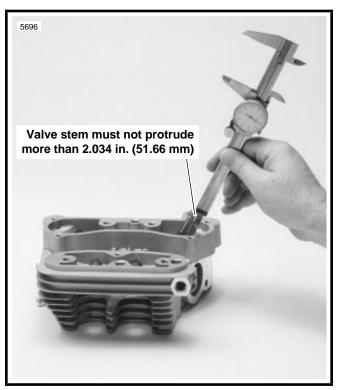
Figure 3-22. Measuring Valve Stem Protrusion
