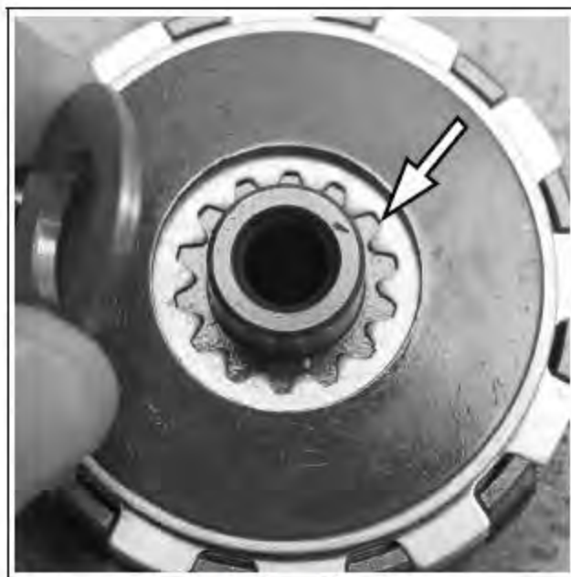
This photo shows how the teeth and splines align together.
