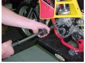
**NOTE:** It is quite common for the older plastic impellers to fall off the end of the shaft during this step of the process if that is the case, then follow the steps at the end of this section to remove the seal and impeller.
