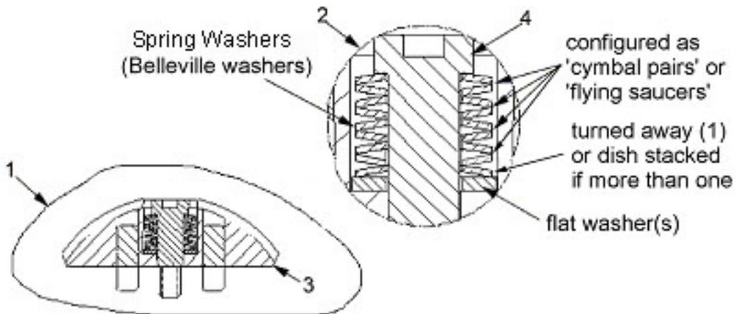
**Figure 32 Some configuration of clutch spring stack.** Each 'spring' stack contains multiple springs (Belleville washers) - arranged into three, four, or five 'flying saucers', or turned away against the flat washer(s). Shown is the 4 ½ stack.
