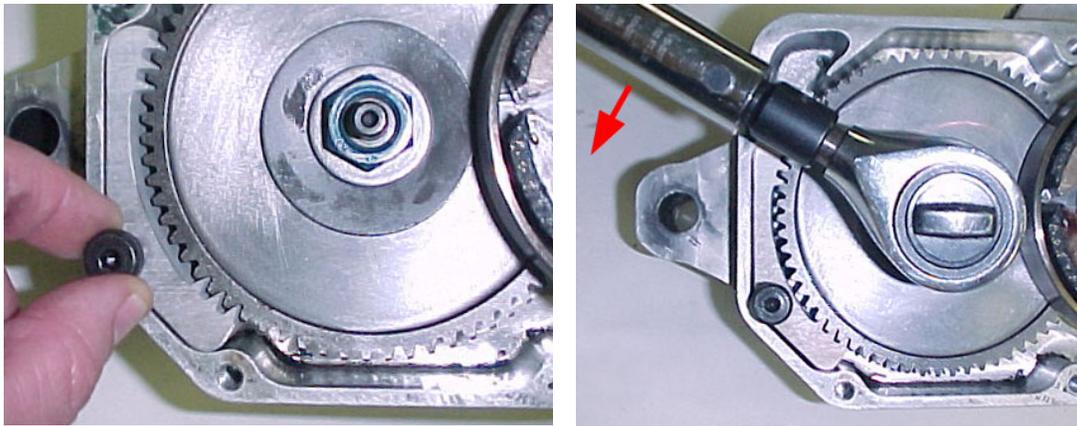
Using a beam style torque wrench, turn the torque wrench counter clockwise and observe the torque measurement when the shaft slips relative to the gear. Using a preset value torque wrench, adjust the setting **55 ft-lb (75 Nm)** and observe whether the wrench clicks first or the shaft slips. If the shaft slips first, the slip torque is below 55 ft-lb and the CFD needs servicing. If the wrench clicks first, the CFD is of acceptable value.
