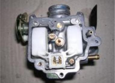
A photograph of the final carburetor assembly, showing the float chamber and various jets and screws.                    |
