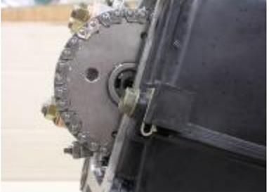
A close-up photograph of the fly wheel and cam sprocket area. The fly wheel is a large, circular metal disc with a 'T' mark. The cam sprocket is a smaller gear with an 'O' hole. The image shows the fly wheel being rotated to align the 'T' mark with an index mark on the crankcase cover.                                                                                                    |
