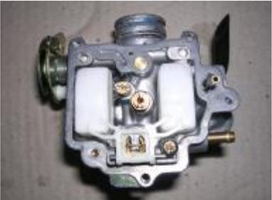
A photograph of a carburetor assembly, showing the float chamber and various jets and screws.                              |
