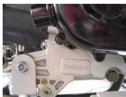
The engine serial number is stamped on the left bottom crankcase.
