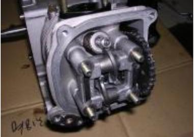
A photograph showing the camshaft holder assembly, which is a silver metal component with a camshaft and a timing chain. The assembly is resting on a cardboard surface.                                                                                                                                                                                                                          |
