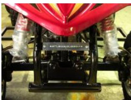
The frame serial number is stamped on the forward part of the frame.
