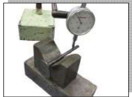
Valve head radial runout
