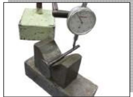
Valve head radial runout
