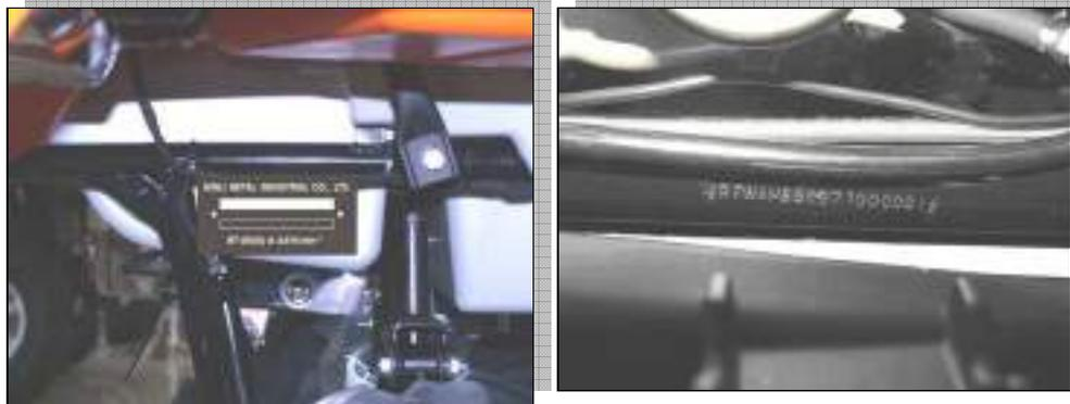
Whenever corresponding with DINLI about a particular issue, the engine number and serial number are important for vehicle identification.
