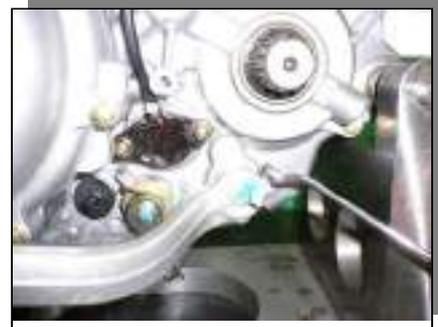
**Apply grease onto front and rear surfaces of Sprocket 14T, and install it in position.**
