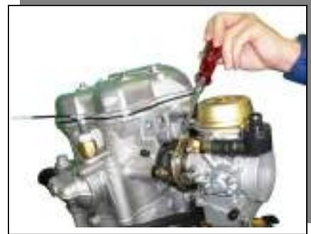
**Fit Shift Pedal with the markings aligned.**
