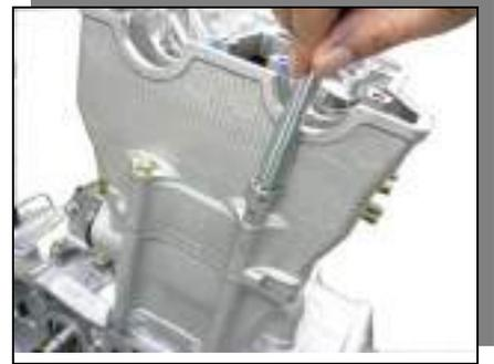
**Install Chain Lever with pivot bolt.**
