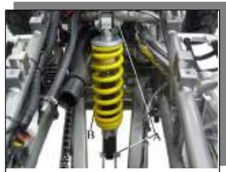
**Rear Shock Absorber Preload Adjustment**
