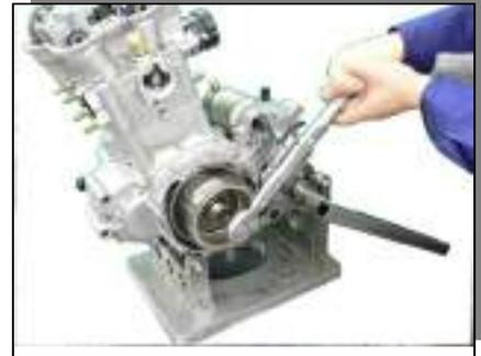
Tightening Torque: 150 – 170 N-m
