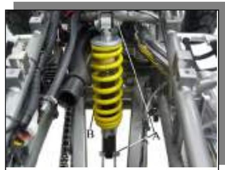
**Rear Shock Absorber Preload Adjustment**
