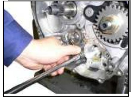
**Assembly Oil Pump Assy. as shown in the illustration in advance.**
