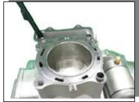
**Assemble Cylinder Head as shown in the illustration**
