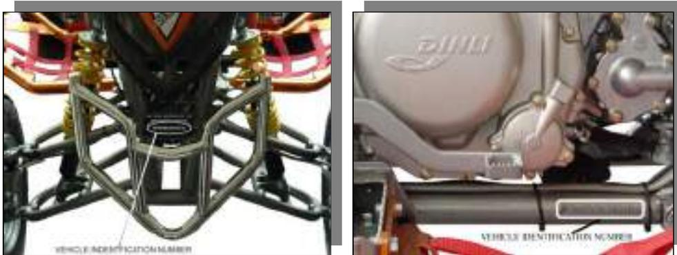
Whenever corresponding with DINLI about a particular issues, the engine number and serial number are important for vehicle identification.
