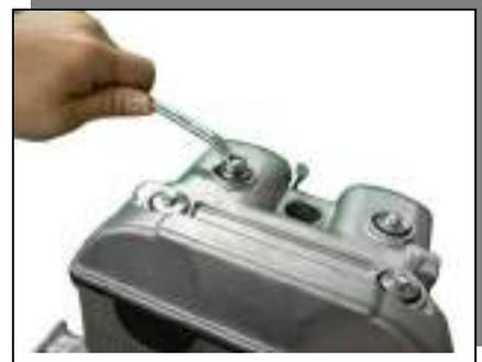
**Install carburetor onto Adapter.**
