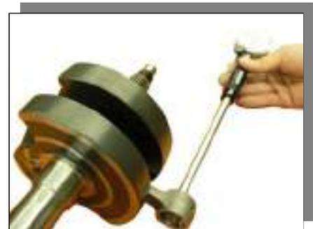
**Clearance between small end ID and Piston Pin OD**
