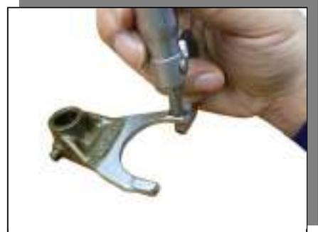
**Clearance between Shift Fork and groove**
