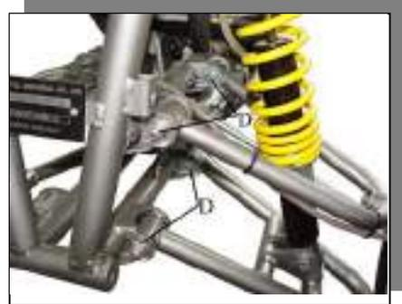
**Suspension Arm Disassembly**
