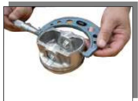
**Clearance between Piston and Cylinder**
