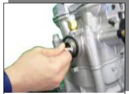
**Install Thermo Switch with the TB #1344 applied to threads.**
