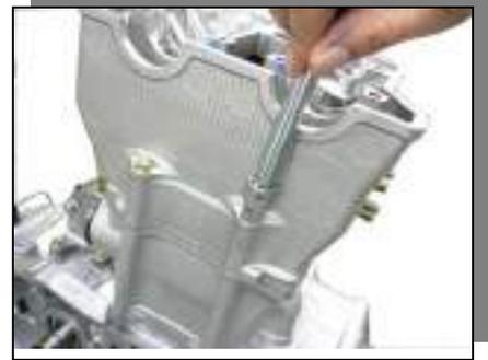
**Install Chain Lever with pivot bolt.**
