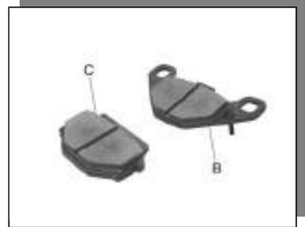
**Torque - Pad Mounting Bolts: 18N-m(1.8kg-m,13.0ft-lb)**
