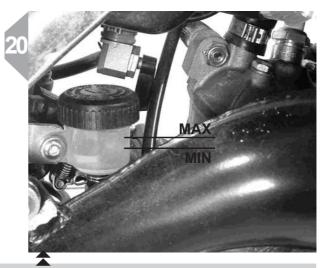
Rear brake fluid - Checking The level is correct if it falls within the min and max marks on the tank. If the level is below the min. mark, top up with the recommended brake fluid.
