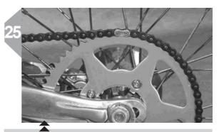
Master link - Checking The master link of the chain has an elastic locking clip. As shown in the photo, place the closed part of the clip in the direction of the chain rotation.
