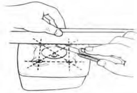
If the largest reading at any portion of the straightedge exceeds the limit, rework the surface by rubbing it against emery paper laid flat on the surface plate in a lapping manner. The surface must be smooth and perfectly flat in order to secure a tight joint: a leaky joint can be the cause of reduced power output and increased fuel consumption.
