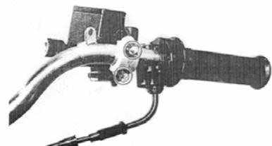
Remove the brake lever and brake switch.
