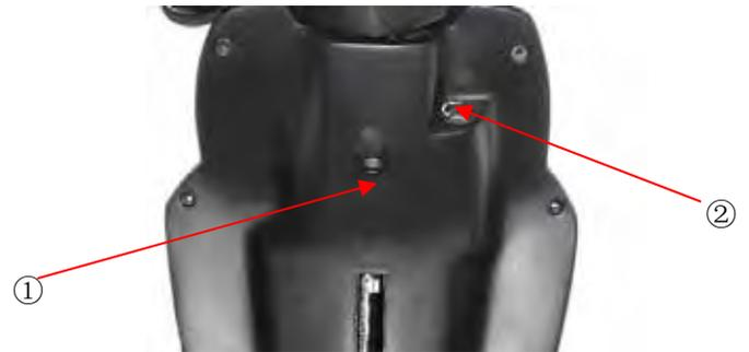
3. remove legshield and pedal by unscrewing the four bolts
