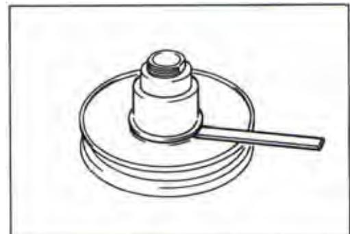
Remove the pins, movable driven face and fixed driven face.
