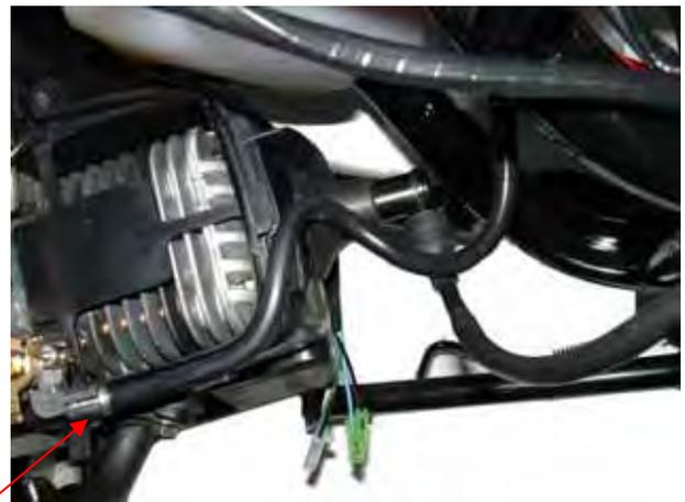
4. Remove rear brake cable adjusting nut
