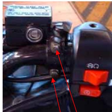
3. Disconnect throttle cable and oil pump cable
