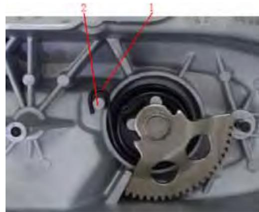
Install starter ratchet wheel and circlip
