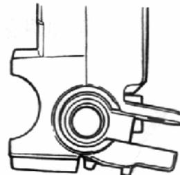
Inspect the piston surface for scratches or other damage.
