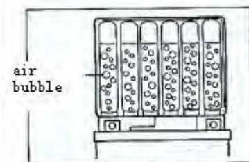
*Test the battery after the filling process. If necessary charge the battery about 20 minutes with the charger.*
