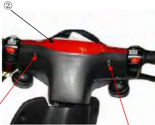
2. Remove master cylinder by removing the bolt ;
