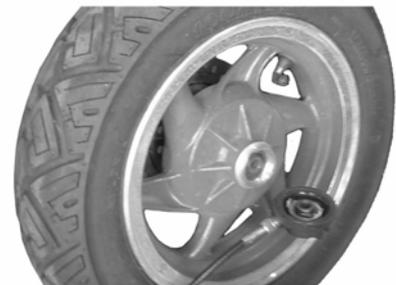
When installing this speedometer gear box, align the two driving pawls with the two recesses of the wheel hub.
