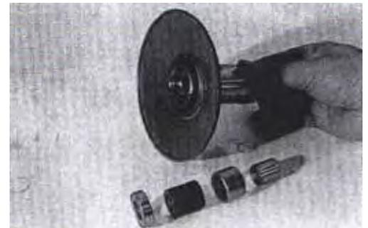
Remove the oil seal from the gearcase cover with the special tool.
