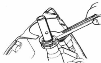
*install handlebar and tighten the screw and*
