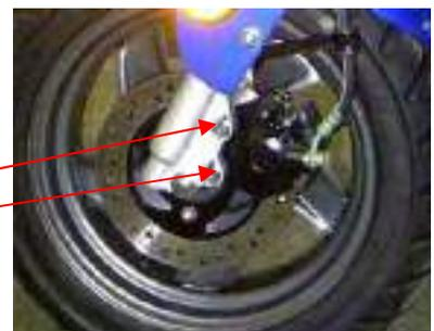
· Remove the brake pads.
