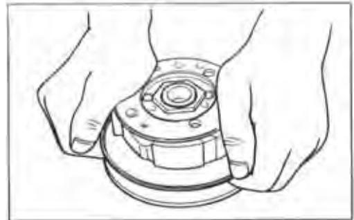
**WARNING:** Gradually back off the clutch shoe assy, pressed down by hands to counter the clutch sparing load. Releasing the hand suddenly may cause the following parts to fly apart.
