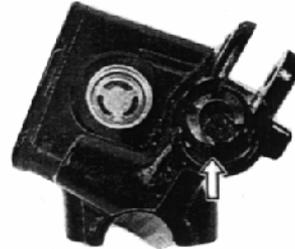
Remove the piston/primary cup with return spring.
