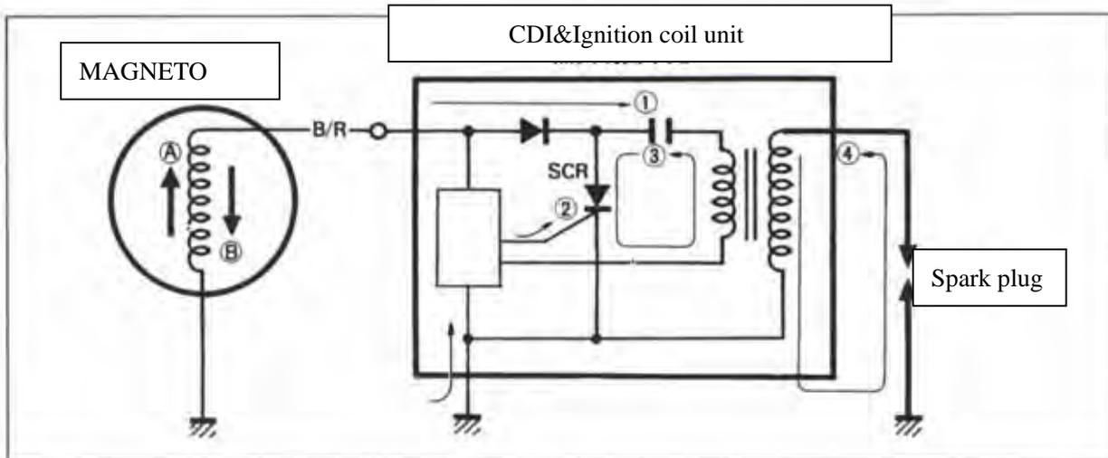
The ignition system consists of a flywheel magneto, a CDI&Ignition coil unit and a spark plug.
