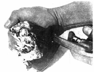
· Place a rag over the piston to prevent popping up. Force out the piston with an air gun.
