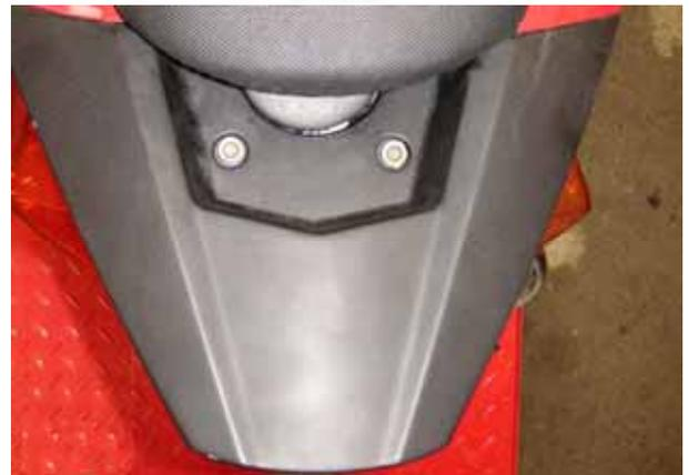
3. unlock oil pump cap and remove it, two tapping screw are exposed, remove them; remove tapping screw; then remove side cover
