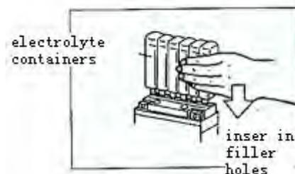
Make sure air bubbles are coming up each electrolyte container, and leave in the position for about more than 20 minutes.
