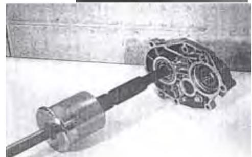
Remove left crankcase oil seal
