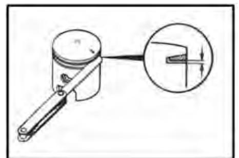
Fix the piston ring in the piston ring groove, measure the ring side clearance with the thickness gauge while matching the sliding surface of piston and ring.
