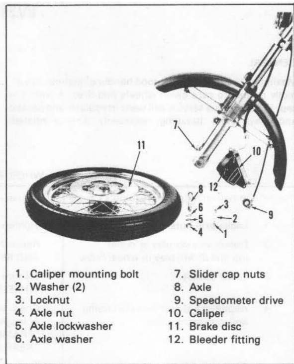
Figure 2-7. Front Wheel Removal (1974 to 1977)
