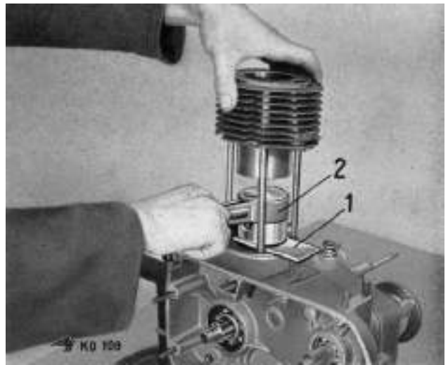
9 Fitting the cylinder
