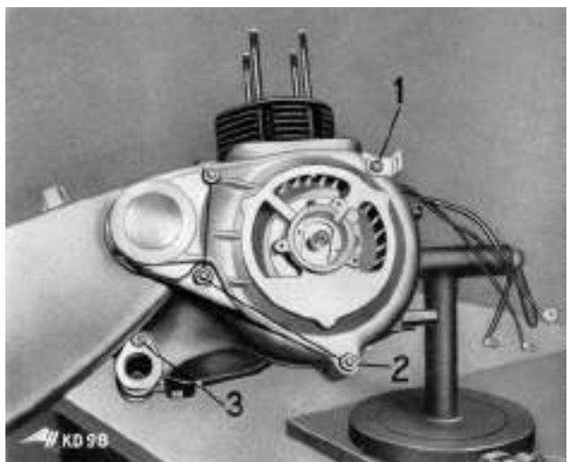
57 Fitting fan housing
