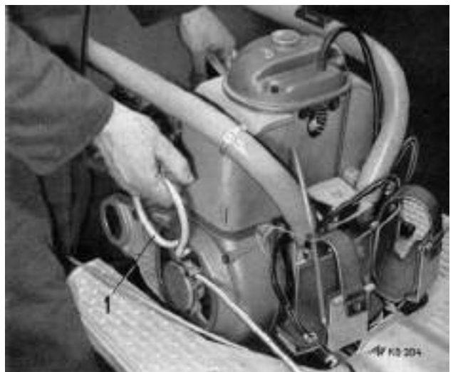
6 Lifting the engine out
