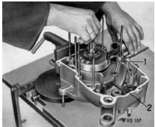
65 Fitting the crankshaft
