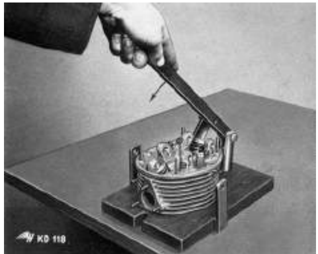
15 Dismantling cylinder head
