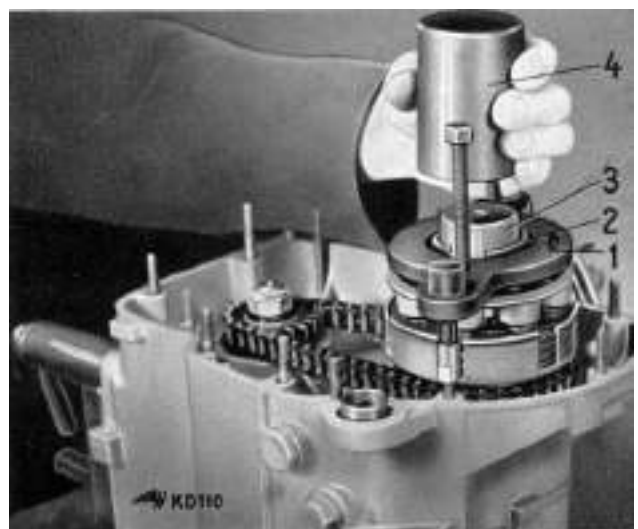
28 Fitting the clutch
