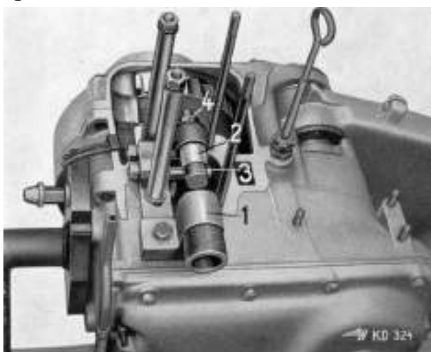
13 Inserting connecting rod bush
