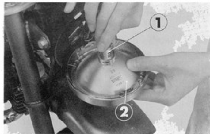
① Headlight socket ② Reflector
