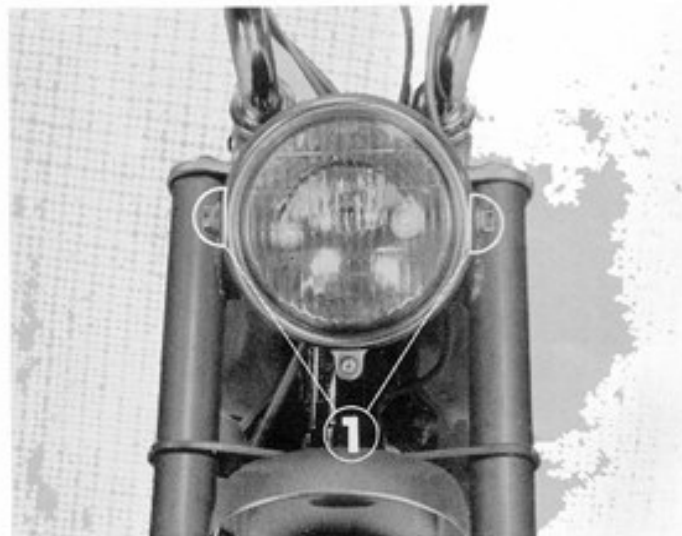
① Headlight mounting bolts
