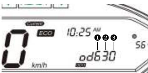
After setting the minute of the time, press the adjustment button again for a long time. The hundreds place ① of the front tire diameter will start flashing, and the short press will cycle between 0 and 9.
