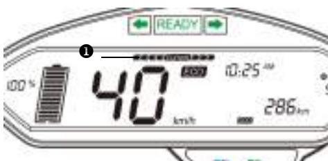
The current indication ① displays the real-time current in the form of a status bar. You can roughly determine the current real-time current through the status bar
