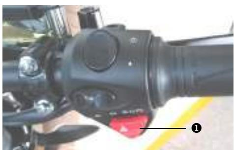
When the button ① is pressed, the turning lights flash to warn other drivers of situations, which include stop or park under emergency conditions.
