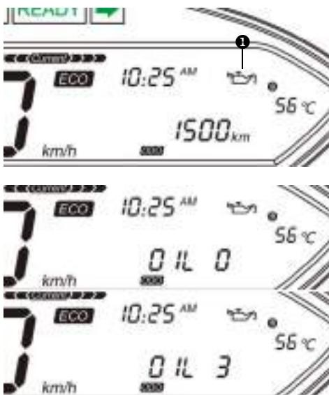
According to the mileage and time of your trip, the system will automatically remind you that gear oil in the reduction gearbox should be replaced. You can manually clear the reminder after changing the oil, or our service personnel can clear it for you.
