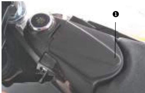
The charging dock is in front of the seat. Press the back of the charging cover to open it.
