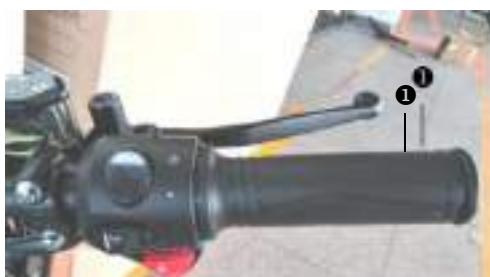
The throttle grip 1 is fitted on the right side of the handlebar.
