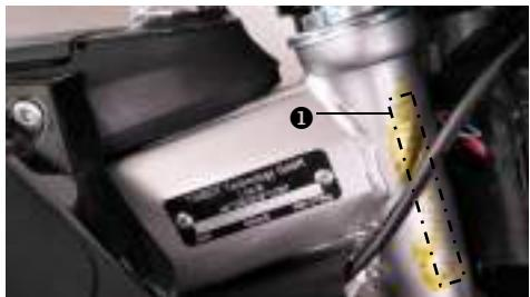
The chassis number ① is stamped on the right side of the steering head.
