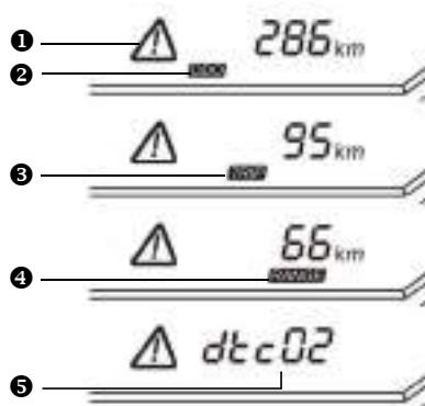
When the error code indicator ① turns on, it indicates a fault in the motorcycle. The error code is displayed in the odometer.
