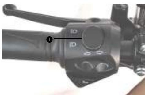
The headlight high/low beam ① switch is on the left handle switch.
