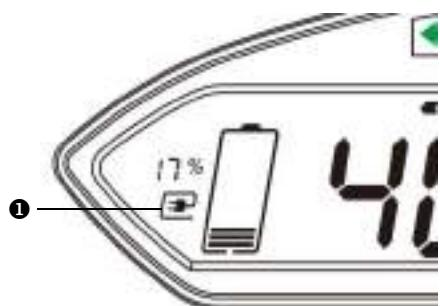
This charging indicator symbol ① display when the battery is charging.
