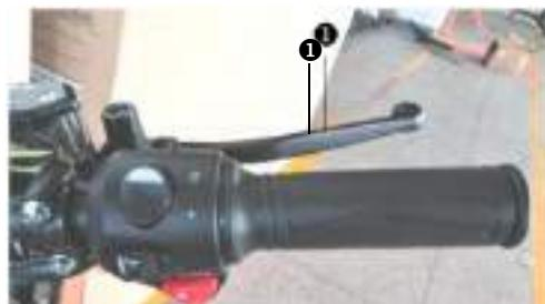
The front brake handle 1 is fitted on the right side of the handlebar.
