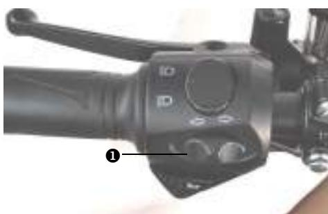
The steering lamp switch ① is on the left handle switch.
