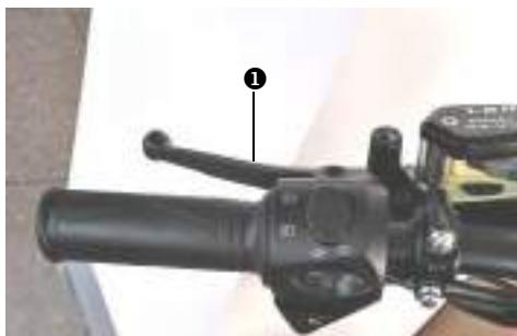
The rear brake lever 1 is fitted on the left side of the handlebar.
