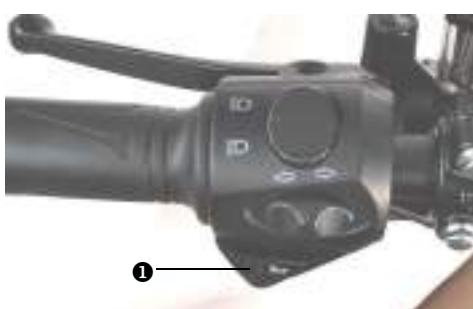
When the key is in the ON position, the horn sounds when the button ① is pressed. The horn can be used to warn pedestrians or other motorists of your presence.
