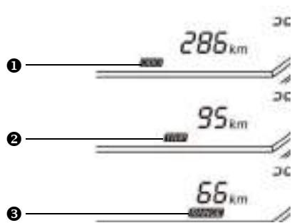
According to the mileage and time of your trip, the system will automatically remind you that gear oil in the reduction gearbox should be replaced. You can manually clear the reminder after changing the oil, or our service personnel can clear it for you.
