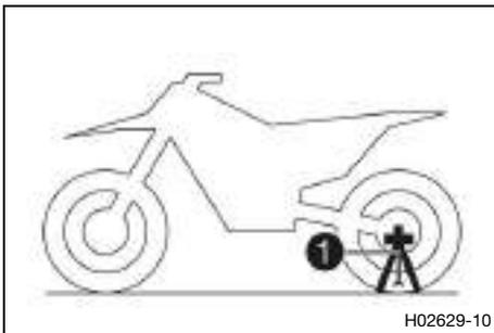
Support for plug-in stand **1** is the left side of the wheel spindle. The plug-in stand is used to park the motorcycle. The plug-in stand is used as a fork locker when transporting the motorcycle.
