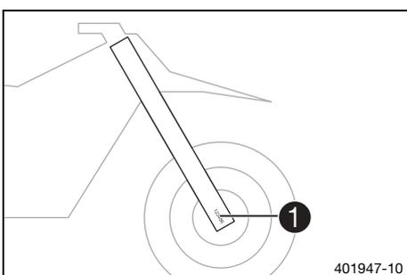
The fork part number ❶ is stamped on the inside of the axle clamp.
