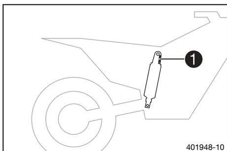
The shock absorber article number **1** is stamped on the top of the shock absorber above the adjusting ring towards the engine side.
