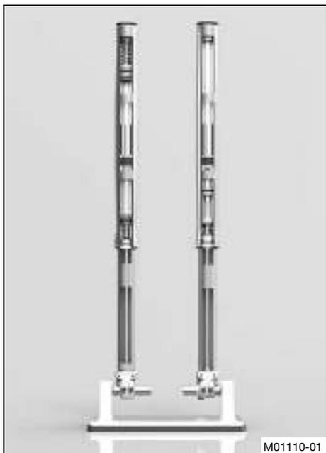
Air suspension **WP Suspension AER 48** is used in the fork. In this system, suspension is located in the left fork leg and damping in the right fork leg.
