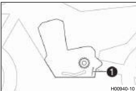
The engine number ❶ is stamped on the left side of the engine.
