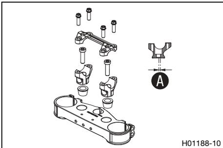
The holes on the handlebar supports are placed at a distance of **A** from the center.
