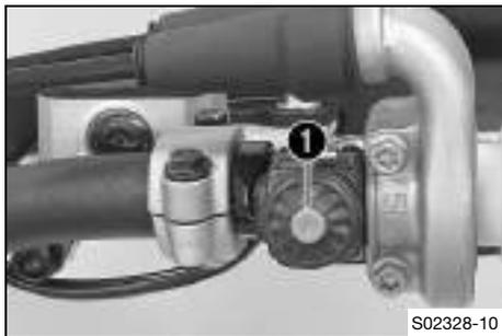
Electric starter button **1** is fitted on the right side of the handlebar.
