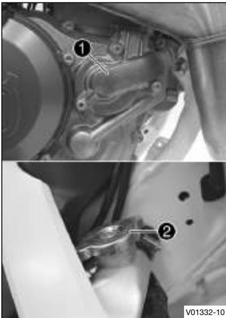
Water pump ① in the engine circulates the coolant. The pressure resulting from the warming of the cooling system is regulated by a valve in radiator cap ②. This ensures that operating the vehicle at the specified coolant temperature will not result in a risk of malfunctions.
