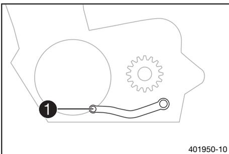
Shift lever **1** is mounted on the left side of the engine.
