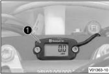
The run hour counter ① is fitted in front of the handlebar. It shows the total number of service hours of the engine. The service hour counter begins counting when the engine is started and stops when the engine is switched off.
