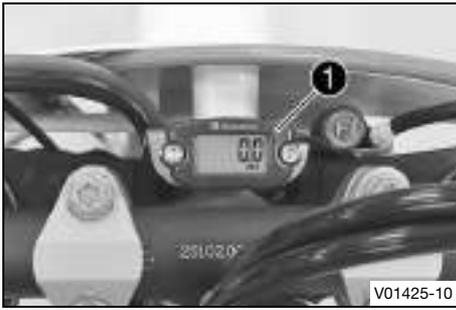
The service hour counter ❶ is fitted in front of the handlebar. It shows the total number of service hours of the engine. The service hour counter begins counting when the engine is started and stops when the engine is switched off.
