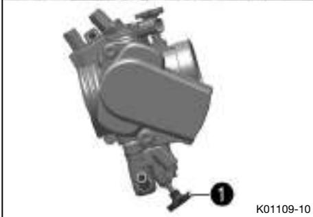
Cold start button **1** is fitted to the bottom of the throttle valve body.
