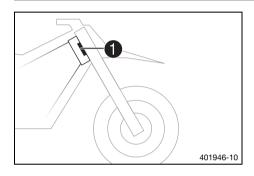
Type label 1 is fixed to the front of the steering head.
