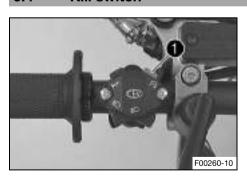
Kill switch is fitted on the left side of the handlebar.
