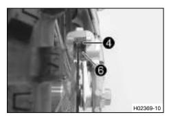
Check that leaf spring 4 in the brake caliper and sliding plate 6 in the brake caliper support are seated correctly.
