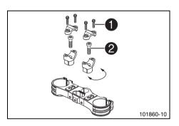
Remove screws 1. Take off the handlebar clamps. Take off the handlebar and lay it to one side.
