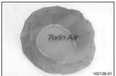
Mount a sand cover on the air filter.
