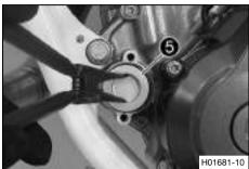
Pull oil filter 5 out of the oil filter housing.
