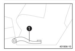
The foot brake lever **1** is attached in front of the right footrest. The foot brake lever is used to activate the rear brake.
