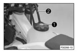
Fit the filler cap and turn clockwise until release button locks in place.
