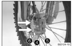
Manually press the brake caliper toward the brake disc to push back the brake pistons. Ensure that brake fluid does not flow out of the brake fluid reservoir, if necessary extract excess
