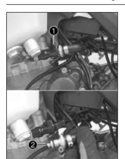
Clean plug-in connection 1 of the fuel line thoroughly with compressed air.
