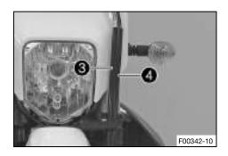
Position brake line 3 and wiring harness 4 in the brake line guide.
