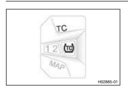
Press button TC to switch the traction control on or off. Guideline
