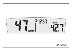
Press one of the buttons until **DST** appears on the combination instrument.
