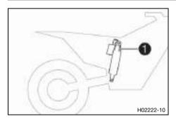
Shock absorber article number 1 is stamped on the top of the shock absorber above the adjusting ring towards the engine side.
