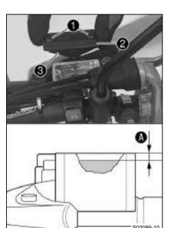
Correct the brake fluid quantity to level A.
