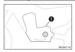
Engine number **1** is embossed on the left side of the engine over the engine sprocket.
