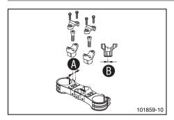
On the upper triple clamp, there are two holes at a distance of **A** to each other.
