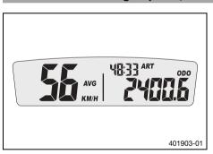
Press one of the buttons until AVG, ART and ODO appear on the combination instrument.
