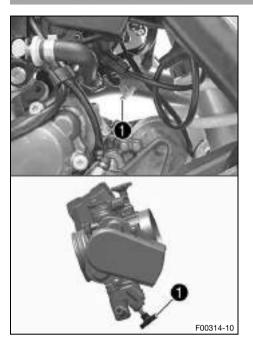
The cold start button **1** is fitted on the bottom of the throttle valve body.
