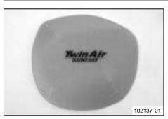
Fit a rain cover on the air filter.
