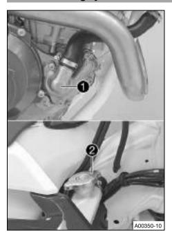
Water pump 1 in the engine ensures forced circulation of the coolant.
