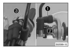
Position half-shells (3), mount and tighten screws (2).
