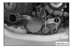
Mount and tighten screw plug 2 with the O-ring. Guideline
