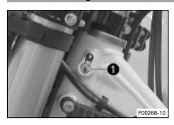
Steering lock is fitted on the left side of the steering head. The steering lock is used to lock the steering. Steering, and therefore riding, is no longer possible.
