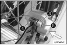
Press the brake caliper onto the brake disc by hand to push back the brake piston and ensure that brake fluid does not flow out of the brake fluid reservoir, extract it if necessary.
