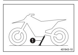
The side stand 1 is attached to the left side of the vehicle.
