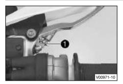
Adjust the basic position of the hand brake lever to your hand size by turning adjusting screw 1.
