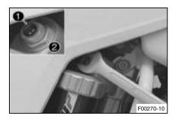
Using an open end wrench, turn adjusting screw clockwise all the way.
