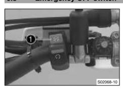
The emergency OFF switch 1 is fitted on the right side of the handlebar.
