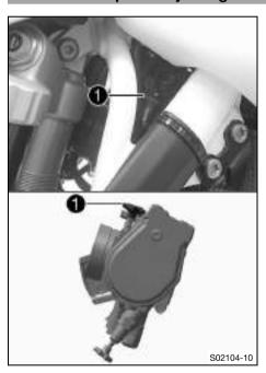
The idle setting of the throttle valve body has a big influence on the vehicle's starting behavior, on stable idling, and on vehicle response when the throttle is opened.
