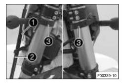
Detach plug-in connectors 4 and take off the headlight mask with the headlight.
