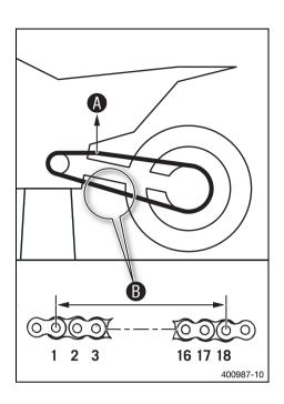
Pull at the top part of the chain with the specified weight **(A)**. Guideline
