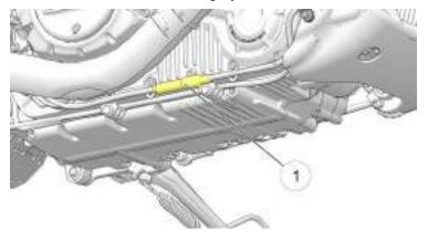
3. While holding the cable, tighten the adjuster lock nut securely.
