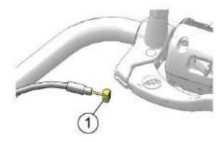
3. Reconnect the cable and adjust freeplay as needed.
