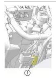
The standard fuse box is located under the seat. This fuse box houses all standard service fuses and the automatic circuit breakers. Fuse application and size are provided on a label on the fuse box cover.
