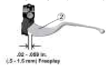
4. Verify that the safety switch activates properly. The engine should not start in gear with the clutch lever ② released.
