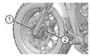
Inspect for debris adhering to the end of the wheel speed sensors (2). If contamination is observed, or if you are unable to visually inspect, slide a thin towel across the face of the sensor between the sensor and the tone ring to remove any potential debris.
