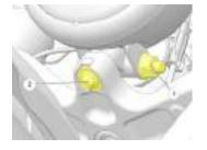
4. Squeeze the bulb retainer ③ and move it away from the bulb. Remove the bulb.
