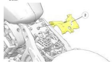
3. Remove the four (4) rear fuel tank bolts ③. Set hardware aside for reassembly.
