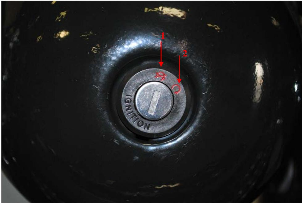
The ignition switch is located at the front of the gas tank on the right side.
