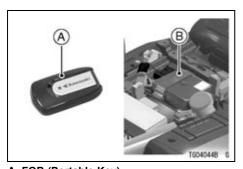
A. FOB (Portable Key) B. KIPASS ECU (Under Seat)
