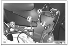
A. Motorcycle Battery Positive (+) Terminal B. From Booster Battery Positive (+) Terminal C. Unpained Metal Surface
