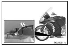
A. Engine Oil Drain Bolt
