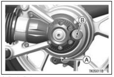
A. Drain Bolt B. Oil Filler Cap
