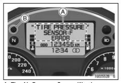
A. Tire Air Pressure Sensor Warning Message (Front Tire)
