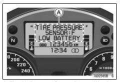
A. Tire Air Pressure Sensor Battery Warning Message (Front Side)
