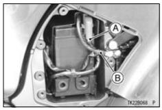
A. Battery (+) Cable B. Battery (-) Cable
