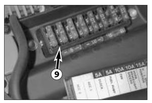
The ACC 1 and ACC 2 fuses **9** are not allocated to specific current consumers in the condition at delivery. They are designed for accessory equipment with a maximum current consumption of 5 amperes each. The respective connectors for this equipment are provided under the headlight cover. For more information, contact an authorized KTM workshop.
