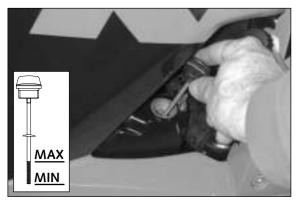
The oil level should fall between the lower end of the oil dipstick (MIN) and the MAX mark.
