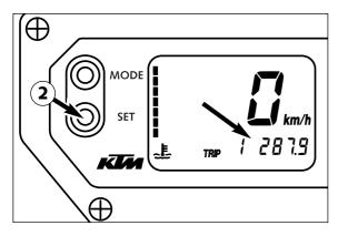
The trip meter 1 runs continuously and counts up to 999.9. It can be used to measure the length of a certain route on a trip or the distance between two refueling stops.
