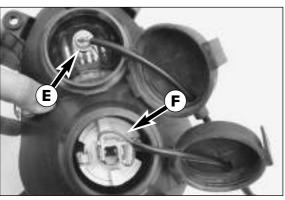
The parking light E is located in the upper part of the headlight in the USA design. • bulb • with high and low beams is mounted in the lower part of the headlight.
