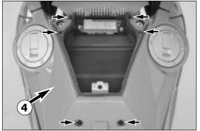
Remove the 6 screws, take off the left panel 5 and disconnect the turn signal cable.
