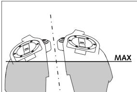
The 950 Adventure has 2 tanks with 1 filler neck each. Fill the right tank first, then the left tank (see drawing for the maximum filling level). If the right tank is filled up to the filler neck, fuel may overflow when the motorcycle is parked on the side stand after refueling when the fuel becomes warm.
