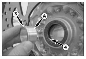
Before remounting the front wheel, clean and grease the shaft seal rings and the bearing surface of the distance bushings and mount the distance bushings (wide distance bushing in the left shaft seal ring). Slightly push back the brake pads with a screwdriver. Position the front wheel against the brake disks according to the direction of travel (see arrow 1).
