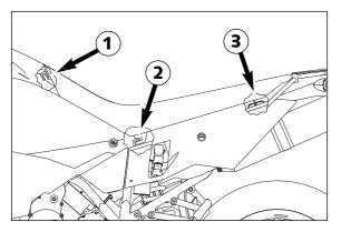
To remount, fit the nose ① of the seat in the front, lower the back while pushing towards the front. Both noses ② should fit into the frame. Insert the catch bolts ③ in the lock housing and push the seat down in the back until you hear the catch bolts snap into place. Check whether the seat is correctly mounted.
