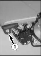
Remove the 3 screws ①, lift the tank approx. 15 mm and carefully tilt to the side. Disconnect the connector from the pickup cable (fuel level) and set the tank down.
