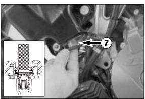
Carefully pull the oil screen out of the oil tank.
