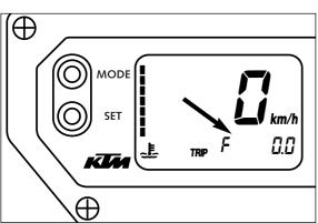
When the fuel level reaches the reserve mark, the display will automatically switch to TRIP F and begin to count (no matter which display mode was active before). At the same time, the fuel warning lamp will start to blink. You will still have enough reserve fuel for aprox 50 kilometers (30 miles). After refueling, it will take approx. 3 minutes for TRIP F to automatically reset to 0 and return to the previous display mode.
