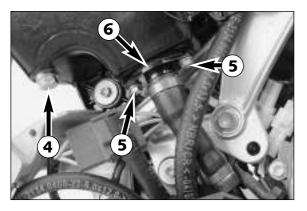
Remove the drain plug **4** on the oil tank and allow the oil to drain into a receptacle. Remove the screws **5** and tilt the oil return valve **6** to the side.
