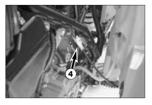
Mount the battery cover and tighten the screws to 25 Nm. Mount the lower screw on the right tank and tighten to 25 Nm.
