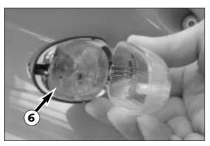
Slightly depress the bulb, turn it approx. 30° counterclockwise and pull it out of the socket.
