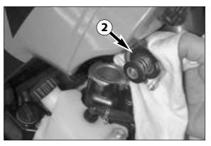
Carefully remove the radiator cap ② with a rag, turning in a counterclockwise direction. The radiator should be completely filled with cooling liquid. No air should be in the radiator.
