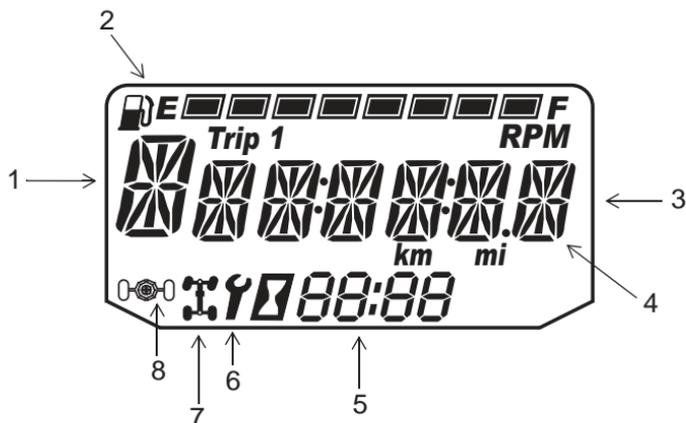
1. **Gear Indicator** - This indicator displays gear shifter position.
