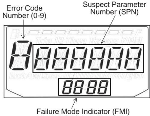
1. If the error codes are not displayed, use the MODE button to toggle until “Ck ENG” displays on the main line of the display.
