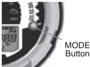
**Tip:** To exit the set-up mode, turn the key off. Wait 5 seconds, then turn the key on. The gauge displays the mode that was displayed prior to setting the units.
