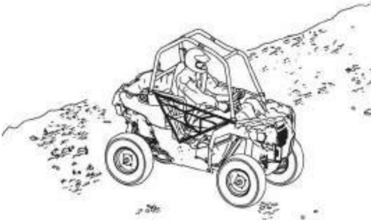
Driving on a sidehill is not recommended. Improper procedure could cause loss of control or rollover. Avoid crossing the side of any hill unless absolutely necessary.
