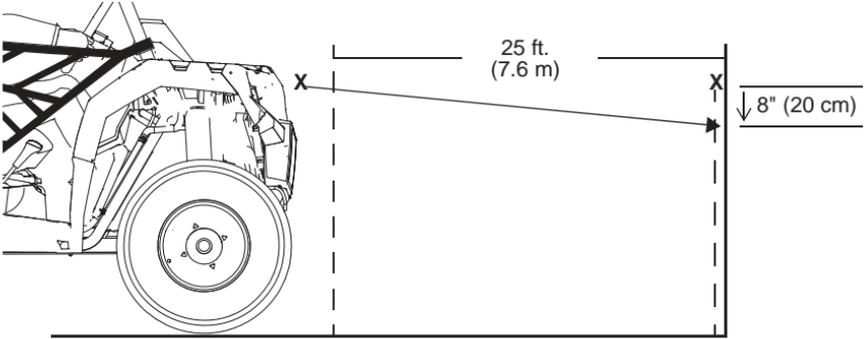
1. Place the vehicle on a level surface with the headlight approximately 25 ft. (7.6 m) from a wall. Place the transmission in PARK.
