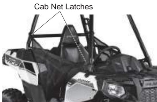
Always inspect cab nets and latches for tightness, wear and damage before each use of the vehicle. Use the strap adjusters to tighten any loose straps. Promptly replace worn or damaged cab nets and latches with new cab nets and latches. Please see your authorized POLARIS dealer.
