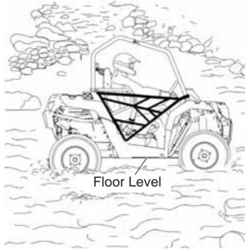
**WARNING!** The large tires on your vehicle may cause the vehicle to float in deep or fast-flowing water, which could result in loss of traction, loss of control, rollover or accident.
