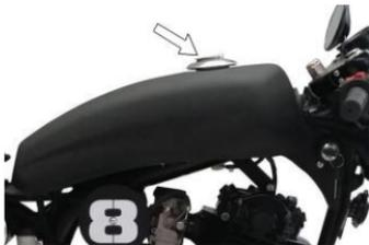
To open the fuel tank cap, insert the key and turn it clockwise. Then, the fuel tank cap can be removed together with the key. To replace the cap, align the arrow on the cap and press the cap, together with the key, into the fuel tank cap hole until a click sound is heard. Then, remove the key.
