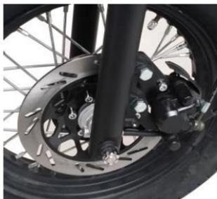
It is essential to check the front and rear brake rotors to make sure they are not below the minimum thickness. If wear exceeds the mark, the brake rotor and pads shall be replaced with new ones.
