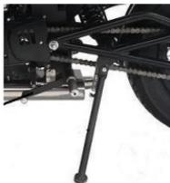
The vehicle is equipped with a side stand.
