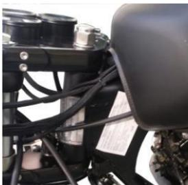
Chassis number (or VIN code) is on the steering stem frame tube. Engine number is on the lower left side of the crankcase. Metal nameplate is on the riser pipe of chassis, showing the main technical parameters, manufacturer and date of production of the motorcycle.
