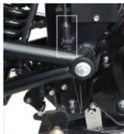
The rear brake light switch is located at the right side of
