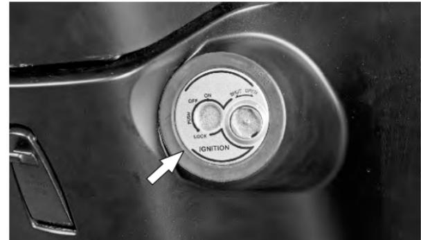
To lock the steering, turn the handle bar all the way to the 'left' or 'right'. Push the key in and turn it to the 'LOCK' position and take out. All the electrical circuits are turned 'OFF' in this position. Safety shutter can be closed in the reverse order of opening. Insert the key into the lock and turn it to 'OFF' or 'ON' position to unlock the steering.
