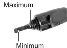
5. If the oil is less than the minimum level, add 'TVS TRU4 PREMIUM' 4T oil upto the maximum level mark.
