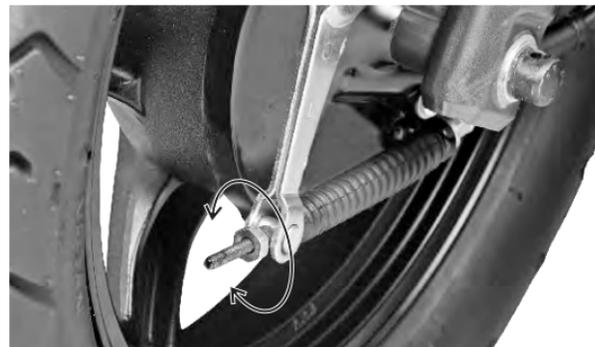
4. Turn the adjuster nut in clockwise direction for reducing the free play or in anti-clockwise direction for increasing the free play.
