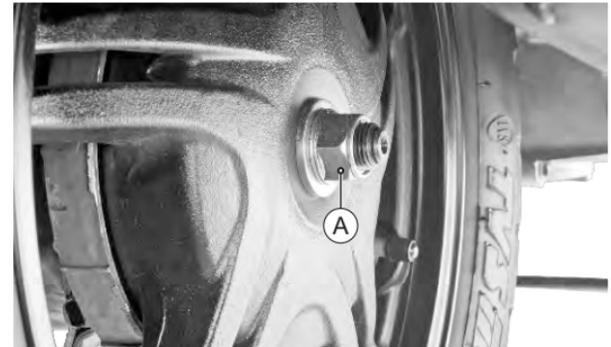
4. Reassemble the wheel in the reverse order of removal. Hold the rear brake firmly while re-tightening the mounting nut for easy locking of wheel.
