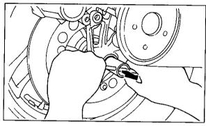
Move the wheel to the right to separate it from the final gear case and remove the rear wheel.
