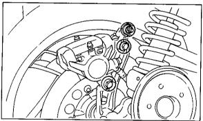
5. While supporting the brake caliper, pull out the rear axle.
