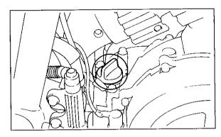
c. Remove the drain plug and drain the oil.
