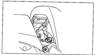
b. Disconnect the leads as shown and remove the ignition coil holding bolts.
