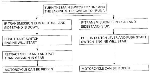
1. Turn the main switch to "ON" and the engine stop switch to "RUN".
