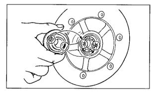
2. Make sure there is enough gap between the brake pads before setting the calipers or discs. 3. Make sure the slot in the speedometer gear unit fits over the stopper on the front fork.
