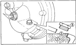
1 Final gear oil 2 Correct oil level 3 Oil filler bolt
