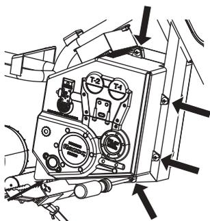
**4** On the opposite side of the charger port, locate and remove the five (5) Phillips screws and lock nuts on the battery cover using a Phillips screwdriver and 8 mm wrench. Separate and remove cover.
