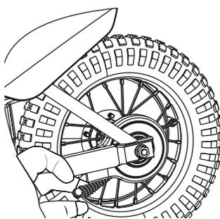
**8** Thread the brake cable through the brake adjuster barrel, through the large spring, and into the small hole in the side of the anchor bolt. Position the cable to the original location (as indicated by the slight cable kink) and tighten securely.
