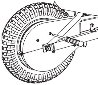
**1** Using a Phillips screwdriver remove the screws on chain guard and remove.
