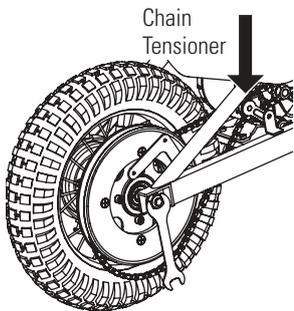
**4** With two (2) 15 mm wrenches, loosen the axle. Push the chain tensioner down to loosen the chain and remove wheel.
