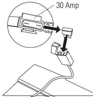
**6** Remove the fuse and replace with a new one of equal amperage. Close the fuse cover and reattach the battery cover, fairing, and plastic cap.
