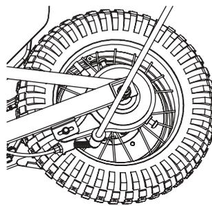
**9** Tighten the cable guide bracket bolt. Tighten the locknuts on the rear axle. Test the brake to verify proper function before riding. Readjust as needed.
