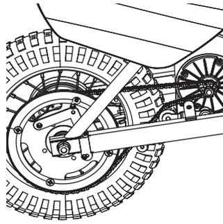
**6** Verify chain is properly installed on each sprocket and tensioner is correctly positioned at the bottom of the chain.
