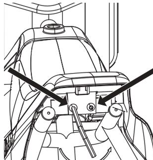
**3** Using a 5 mm Allen wrench, loosen the two (2) bolts underneath the rear of the seat and remove the fairing.
