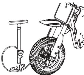
Using a bicycle tire pump equipped for a Schrader valve, inflate both tires to the PSI indicated on the sidewall of the tire.
