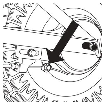
**2** If the brake has too much slack, use a 10 mm wrench to loosen the brake anchor cable for additional adjustment and retighten.
