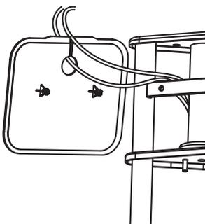
Slip the cables through the slit on the top of the number plate. Align the number plate with the holes on the fork and snap on the number plate.
