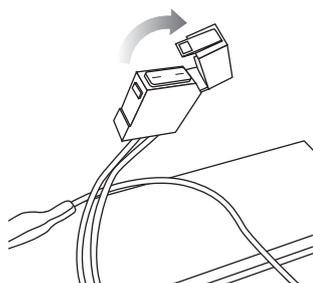
**5** Locate the fuse box attached to the batteries. Open the fuse cover to expose the fuse.
