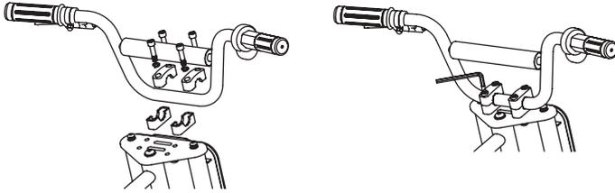
**1** Place the handlebars in the handlebar clamps.
