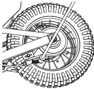
**2** With a 10 mm wrench, loosen the brake cable anchor bolt and disconnect the cable.
