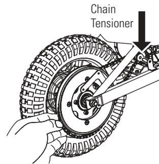
**5** Install the chain onto the rear wheel sprocket. Slip wheel axle into the frame slots. Push the chain tensioner down to create slack in chain. Hand tighten rear axle locknuts.
