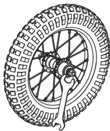
**2** Remove the nuts on both sides of the front axle using a 15 mm wrench then remove the axle safety washers.
