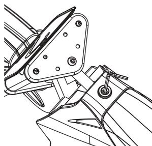
**2** Using a 5 mm Allen wrench, remove the bolt.
