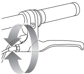
**1** To adjust the tension, thread the brake lever adjuster in or out 1/4 to 1/2 turn until the desired brake adjustment is attained. Most adjustments are complete at this step. If brake still needs further adjustment, proceed to step 2.
