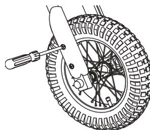
**3** Remove front wheel and install replacement wheel. Re-attach fork covers.
